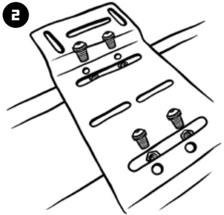
2) Place the mount on top of the bonded washers and insert 8 5/16" bolts. Be sure to include 5/16" lock washers and 5/16" washers on each bolt. Make sure bolts are securely fastened.
