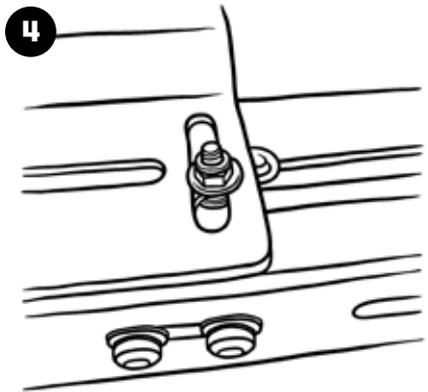
4) Set your tank on top of the platform rack and align the bolts with the slots located on each side of the tank. Insert 4 washers and then place the 4 lock nuts and thread on tightly.
