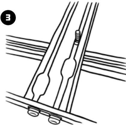
3) Insert 4 carriage bolts into your vehicle's rack by sliding them forward or backward. Make sure they align with the slots in the mounts.
