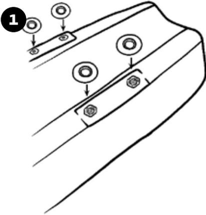
1) Place 8 neoprene rubber bonded sealing washers onto the tank (with the black/rubber side against the tank).
