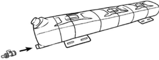
1) Attach the on/off to your tank by threading it on clockwise. Tighten the on/off by the collar, not the body of the valve.
