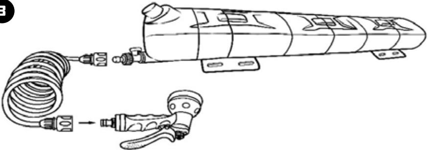
3) Attach the nozzle by pushing in the male quick connect (located on the bottom of the nozzle) to the quick connect at the end of the 16' hose.
