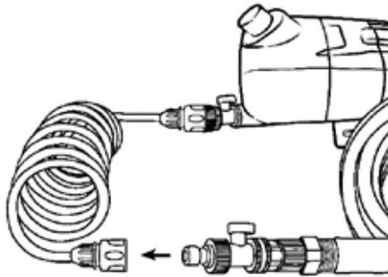
2) To self-pressurize your tank attach the regulator to the end of the provided 16ft hose. Turn the on/off valve on both the tank and the regulator to the on position. The tank will start to fill. It will take approximately 2.5 minutes to fill up. You can also tell it's full by wrapping your hand around the provided hose and wait until you can feel the flow of water stop. Once full make sure both valves are turned to the off position and disconnect the 16ft coil hose from your home garden hose.
