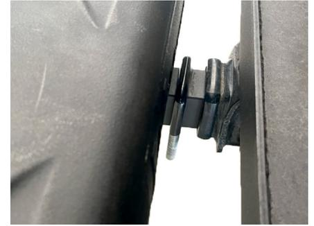
**Step 5:** Slide on the metal plate with the bend facing the front of your vehicle. Please make sure the bent portion is over the lip of your vehicle's hitch adapter. Once this is in place add the washer, lock washer and nut. Tighten the nut with a wrench until the bolt is securely fastened and there is no movement of your tank.
