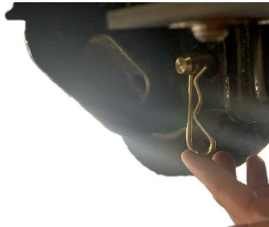
**Step 4:** Attach your hitch stabilizer by sliding the U-bolt over the Weekender hitch bar.
