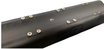
**Step 2:** Place the mount on top of the rubber bonded washers. Make sure the tank's spout is facing the inside of the bumper. Add eight 5/16" washers, eight 5/16" lock washers and eight 5/16"-5/8" bolts (must go in this order, four per side, eight total).
